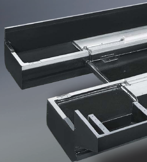
■ The contact area between columns and bed are precisely hand scraped.
