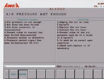
When the alarm appears, the program will display the breakdown cause and a troubleshooting procedure. Users can easily troubleshoot minor problems to save machine shutdown time.
