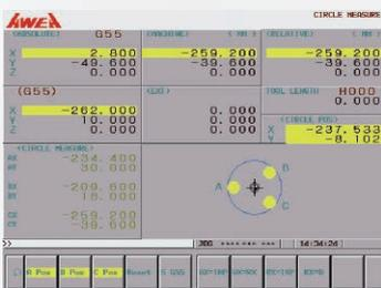
The circular work piece program can calculate the center coordinate of a work piece by measuring point A, B and C coordinates.
