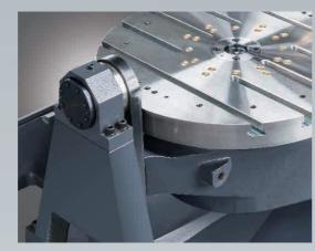
Working table equips super rigidity tailstock support which ensures excellent machining accuracy during heavy loading or unbalancing force on table.
