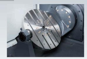
Rotary Working Table Advanced design of rotary table is unilateral driven and supported by both sides of structure to provide outstanding performance and accuracy.
